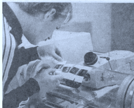
Laser-scanning the slides — one general view and three saucers — is Tim Watson at Pacific Lithographic in South San Francisco. The slides are angled so the saucers can be slipped onto the general view without having to be rotated. From this point on the photos are strictly digital information, no longer an analog of reality.
